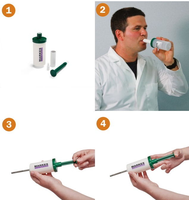
Figure 3: (1) BioVOC-2 components – body with cap, plunger with tip, bung, disposable cardboard mouthpiece and a non-return valve; (2) sample collection; (3) sampling end of a sorbent tube is attached to the tip of the BioVOC-2 body; (4) and the plunger is pushed to transfer the sample to the tube.
