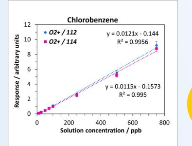
Figure 2. An example calibration curve for the Class 2 residual solvent chlorobenzene, exhibiting excellent linearity across the chosen range.
