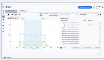
Figure 1. The first step of data processing involves computing a mean intensity across the sample injection profile. The plot illustrates the long, slow injections required for real-time SIFT-MS analysis. In this example, data is collected over the course of 100,000 ms (100 seconds).
