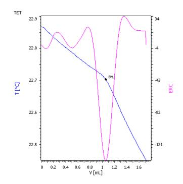
The reliable knowledge of the accurate acid number for crude oil is important for the determination of the price of crude oi. Additionally, by monitoring the acidity of crude oil and the associated process oils unexpected shutdowns can be prevented and thus expensive treatment chemicals preserved. The determination of the acid number in crude oil and various gas oil samples by catalytic thermometric titration is described here.
