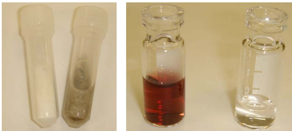
Figure 1: Left: dSPE tubes with 150 mg \text{MgSO}_4 and 150 mg PSA before and after cleanup of 1 mL red wine extract; Right: Red wine extract before and after dSPE cleanup
