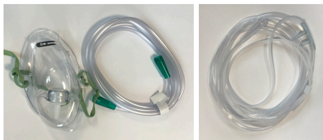
Figure 2: Examples of two of the samples analysed. Left: Face mask supply tubing (the face mask itself was not part of the sampling setup). Right: Nasal cannula.
