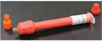
In this study, we investigated the detection limits and the sensitivity of analysis after the ASSET samplers were spiked with a mixture of DBA-isocyanate derivatives representing an air concentration of 5  $\mu$ g/m<sup>3</sup> at an assumed sample volume of 24 L (recommended flow range of the sampler is 0.1-0.25 L/min).
