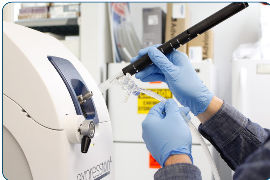
Figure 8: The iASAP, an inert modification developed for the original ASAP, for CMS analysis of air-sensitive samples.
