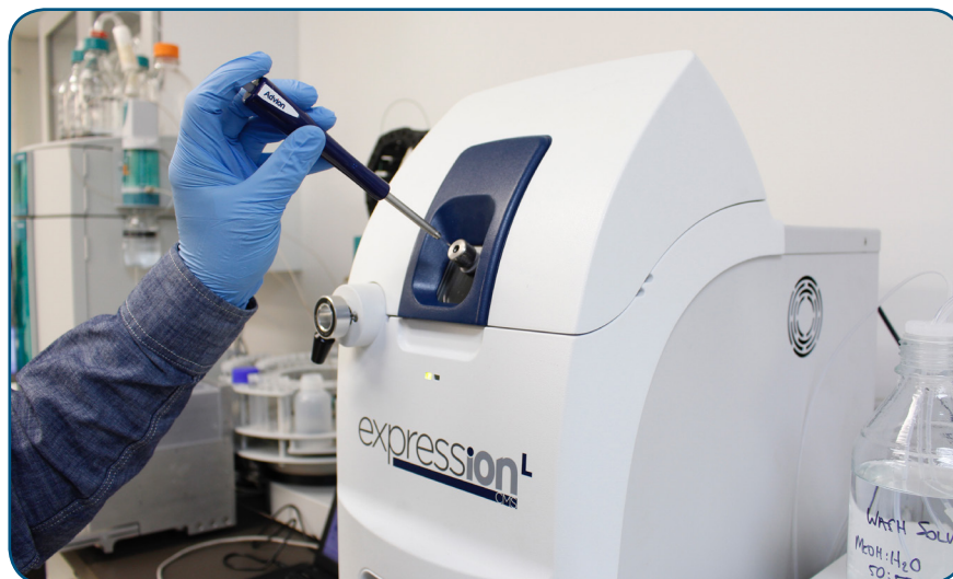
Figure 6: ASAP with sample inserted into the ASAP-enabled APCI ion source of the CMS.
