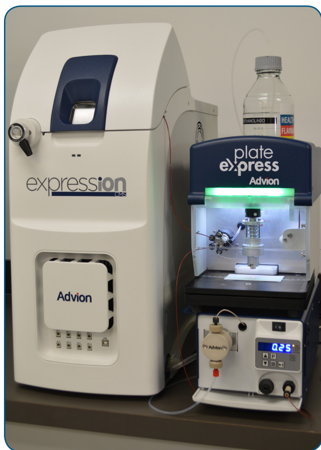
Figure 4: Experimental set up of the CMS and Plate Express.
