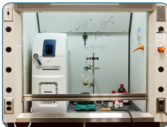
Figure 1: The CMS with reaction equipment directly inside of a fume hood.
