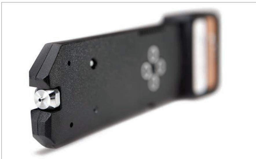
Figure 1. The iKey separation device includes all electronic and fluidic connections, column heater, emitter and ceramic chip inscribed with a 150  $\mu\text{m}$  ID channel packed with 1.7  $\mu\text{m}$  UPLC packing materials.
