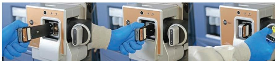
Figure 3. Once the iKey is inserted into the MS source and locked into place, fluidics are connected, the sample is introduced and separation occurs. After separation, the sample travels to a built-in electrospray emitter that converts the liquid stream into an aerosol, ionizes it and introduces it to the MS for further separation.
