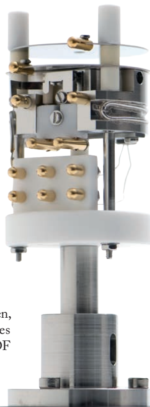
Figure 1. The ion source of the BenchTOF instrument, incorporating technology that ultimately allowed Tandem Ionisation.
