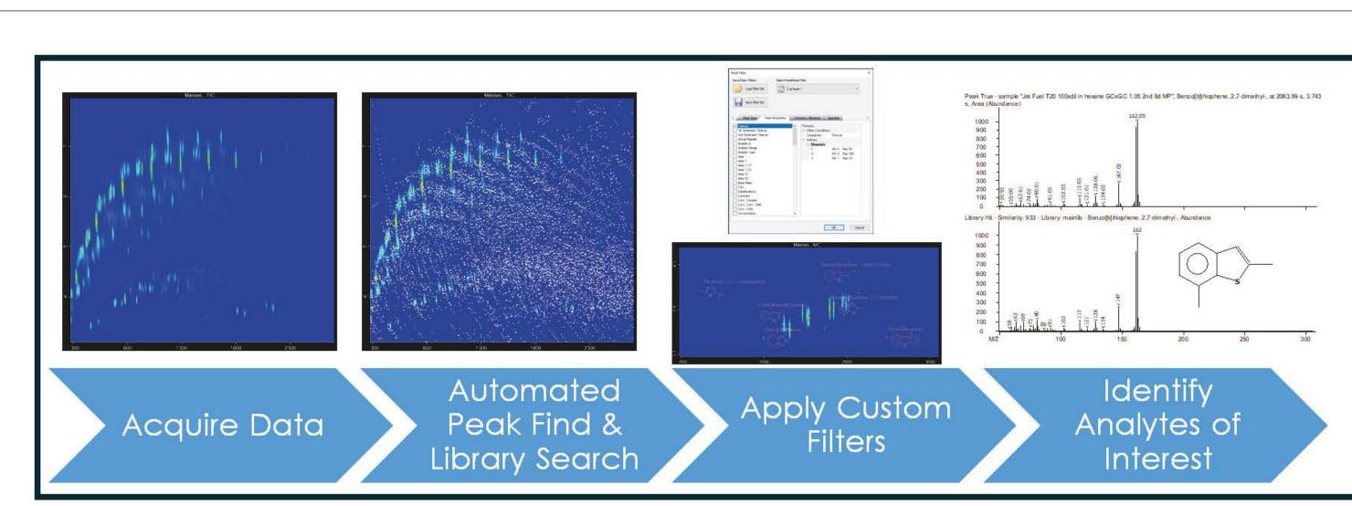
Data processing workflow for semi-targeted analysis of traditional aviation fuel, showing the power of custom peak filtering for narrowing focus to potential analytes of interest.
