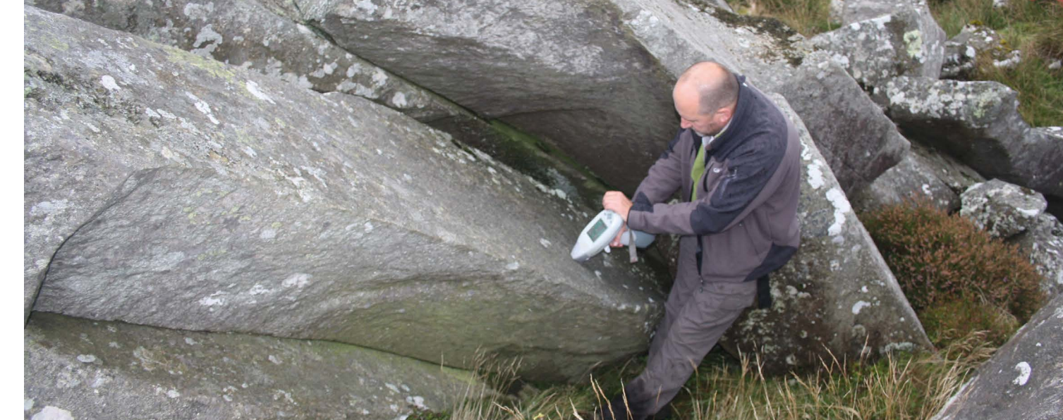
Professor Nick Pearce using a portable XRF to analyse spotted dolerite at Carn Goedog in the Mynydd Preseli, one of the sites identified as a source for spotted dolerite bluestones at Stonehenge. Photo by Richard Bevins.
