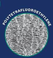
Hydrophobic microporous membrane; suitable for aggressive chemical and air/gas stream filtration
