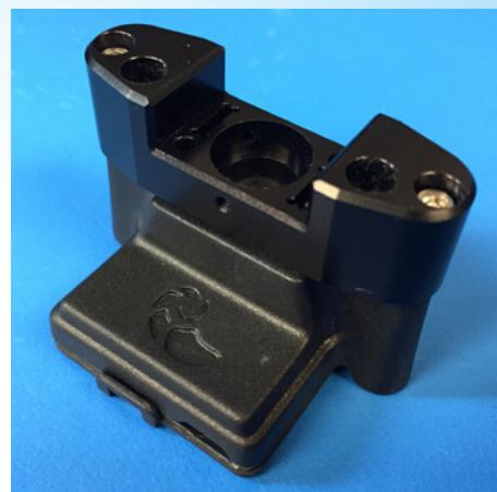
Figure 2: A magnetically mounted diffusing optic helps to provide even illumination of the Spark aperture.
