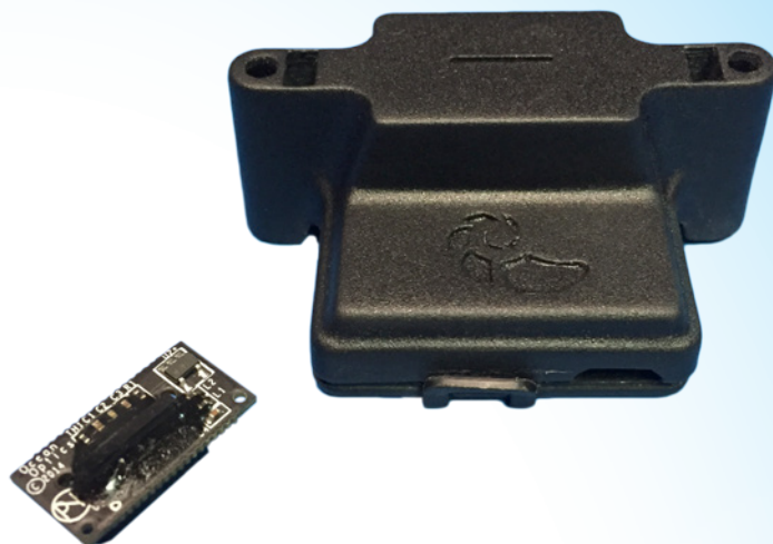
Figure 1: The Spark spectral sensor is available in stand-alone (at right) and embeddable versions.
