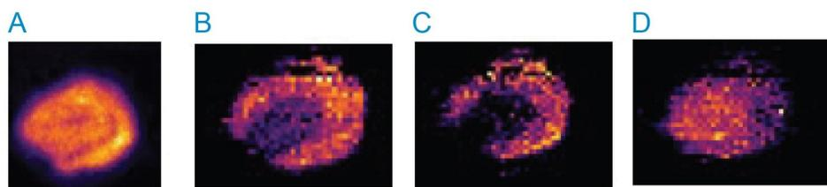
Figure 4. Compound map for  $m/z$  806.55 on the conventional oa-QToF mass spectrometer (A), and individual compound maps for the  $m/z$  806.51007 (B),  $m/z$  806.55829 (C)  $m/z$  806.56909 from the MRT mass spectrometer spectra.
