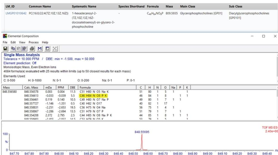
Figure 2. An example elemental composition search within MassLynx software and the corresponding LIPID MAPS<sup>3</sup> database match for the proposed composition from the MRT DESI MSI dataset.
