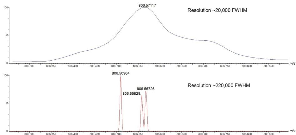
*Figure 3. Representative mass spectra for a narrow  $m/z$  range produced from murine adrenal gland tissue analysis on the conventional oa-QToF mass spectrometer (Top) and the SELECT SERIES MRT Mass Spectrometer (Bottom).*
