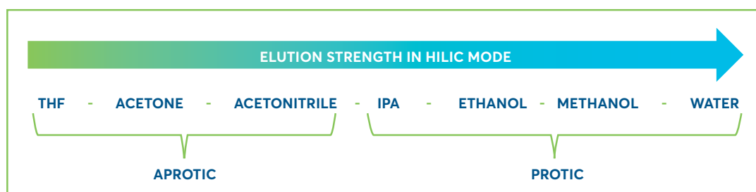
FIGURE 1. Solvent elution strength in HILIC mode.
