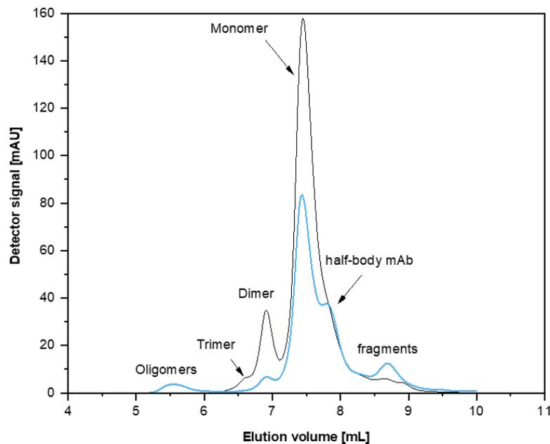
Figure 2: Separation range of the PSS MAB 3 $\mu$ m column. The black curve shows the UV signal of a native antibody and its associates plotted against the elution volume. The blue curve is the elugram of fragmented antibody sample by reduction.
