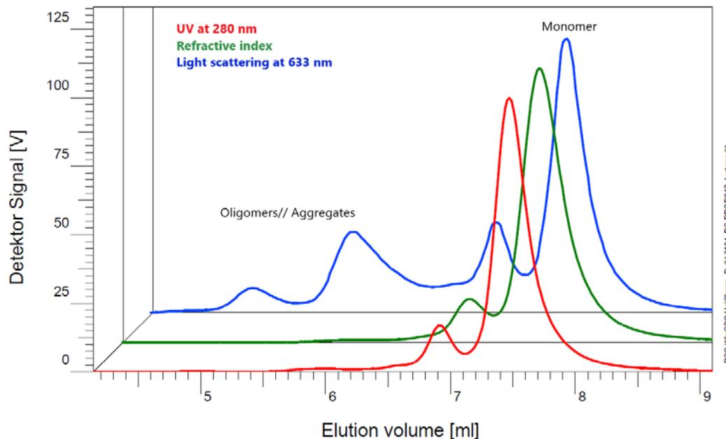
Figure 3: Sensitive analysis of antibody aggregates. The light scattering signal for the antibody associates and higher aggregates is relatively high compared to monomer signal due to molar mass dependency and provides enhanced sensitivity for the detection of high aggregates.
