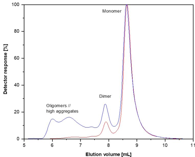
Figure 1: Separation range of the PSS MAB 3 $\mu$ m column. The red curve shows the UV signal of a native antibody and its associates plotted against the elution volume. The blue curve is the elugram of an aggregated antibody sample.
