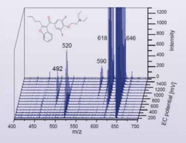
Oxidative "fingerprint" (MS Voltammogram) of Amiodarone (*antiarrhythmic agent*) m/z 646 and its major oxidative metabolites m/z 618, 590, 520 and 492 generated by on-line Electrochemistry-MS using the ROXY EC system equipped with  $\mu$ -PrepCell2.0 and connected to an MS. Total experimental time 15 min.
