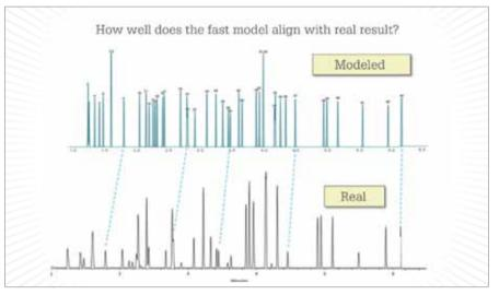
Figure 1. A modeled chromatogram of VOC versus the real result.
