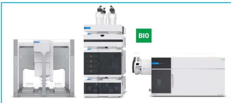
Figure 1: Instruments used for metabolomics workflow - Bravo Sample Prep Platform for reproducible sample prep (left),<sup>2,3</sup> 1290 Infinity II Bio LC (center) has improved peak shape and detection limits for metal-sensitive metabolites, and New 4<sup>th</sup> Generation 6495 LC/TQ (right) uses an ion funnel for low detection limits and low RSDs even when using 0.5 ms dwell times.
