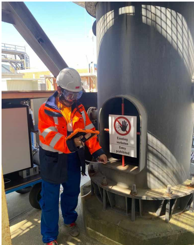
Figure 1: Operator checking a manhole for emissions using the live data streamed to a tablet display from the mobile PTR-TOF instrument. Picture credit: Olin.
