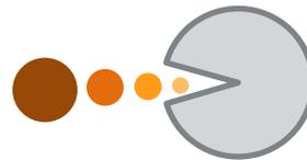
The **smallest compounds** in the sample mixture can enter deep into the pores and have a **long elution time**. The medium-sized components penetrate the pores in some depth and elute separately according to their size.
