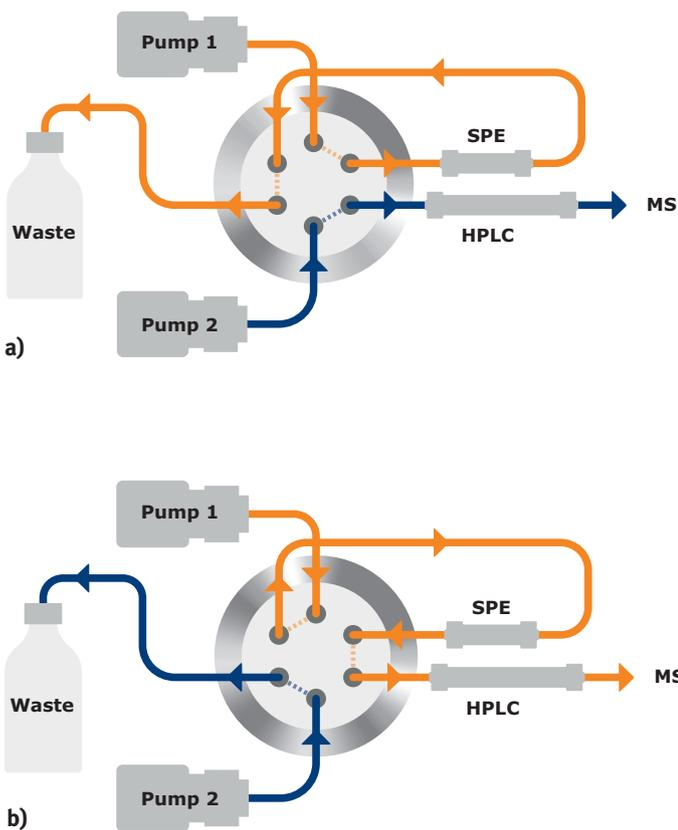
Figure 2. Switching Valve Configuration a) (Top) Valve position 1→2; b) (Bottom) Valve position 1→6
