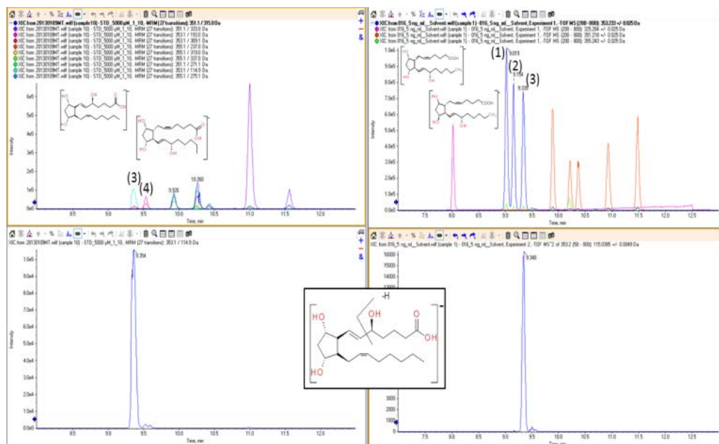
Figure 4. Instrument-dependent specificity. Specificity achieved with different scan techniques on a 4000 QTRAP® System (left side) and on a TripleTOF® 5600+ System (right side).
