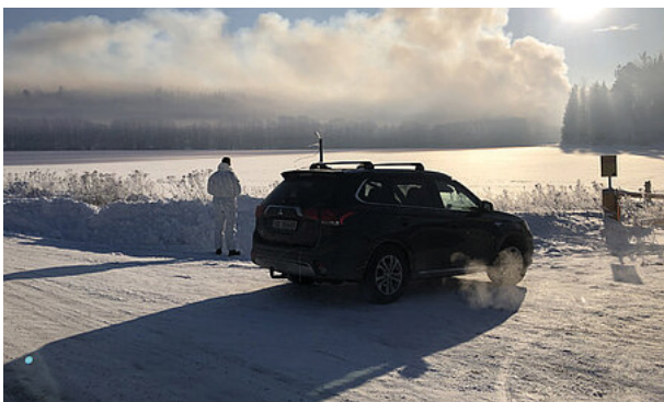
UiO's staff chasing a landfill fire plume, tracking toxic organic gases with their mobile PTR-TOF lab. Image by A. Håland, University of Oslo (UiO).
