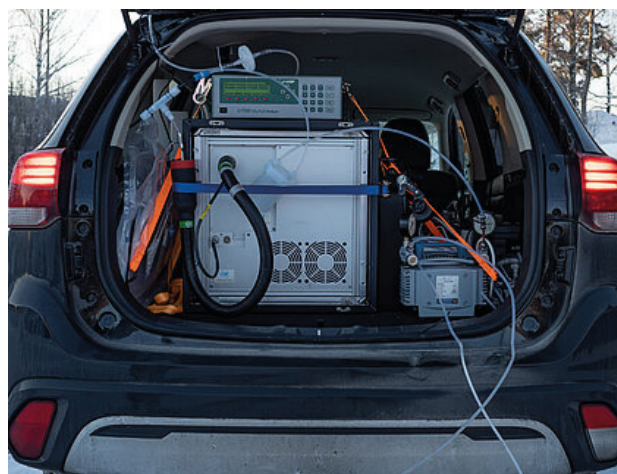
IONICON's PTR-TOF 1000 QB aboard UiO's mobile measurement vehicle.
