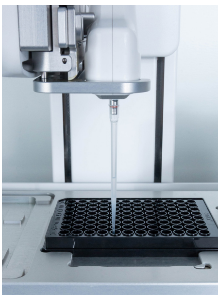
Figure 4: PPC is added by the D-ONE single channel pipetting module.
