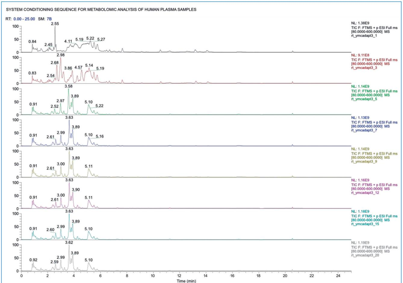
Figure 1: Rapid conditioning of the YMC-Accura Triart Diol-HILIC column and the subsequent excellent reproducibility.
