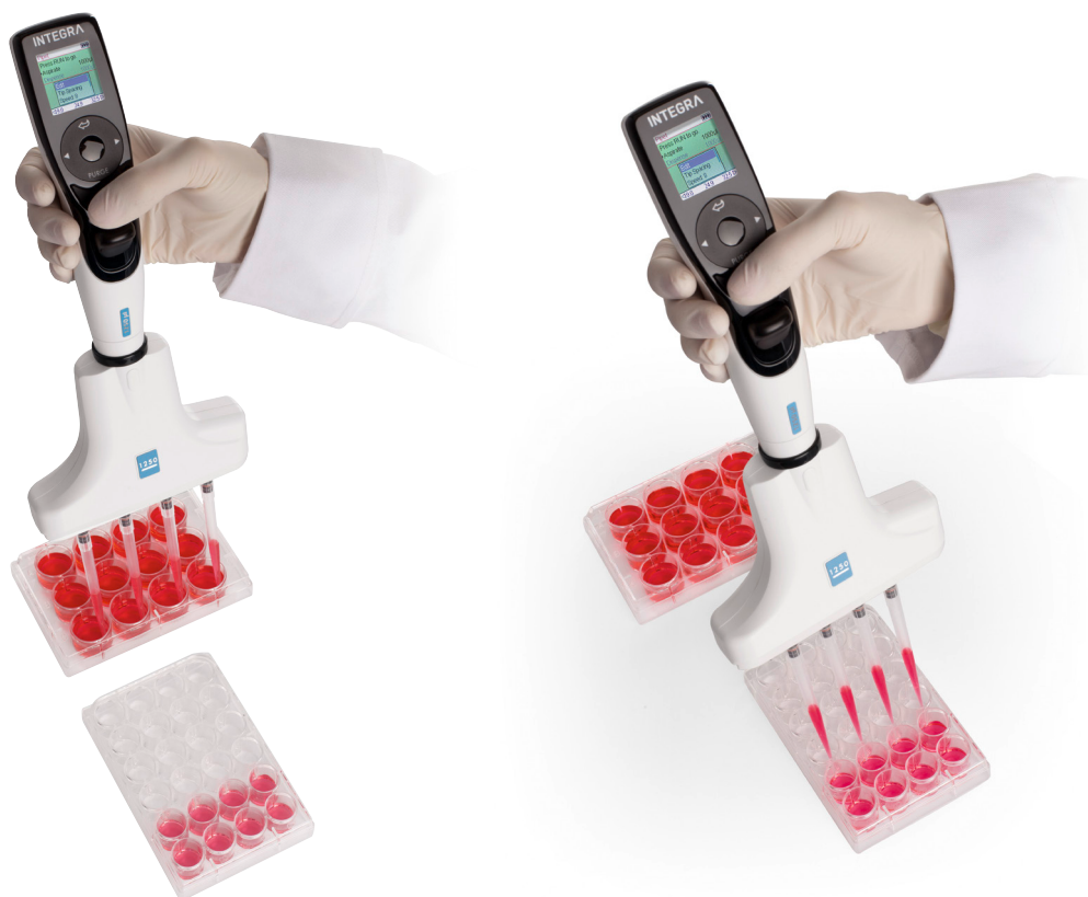
Figure 10: Sample transfer from a 12 well plate to a 24 well plate with a 4 channel VOYAGER 1250 µl adjustable tip spacing pipette.
