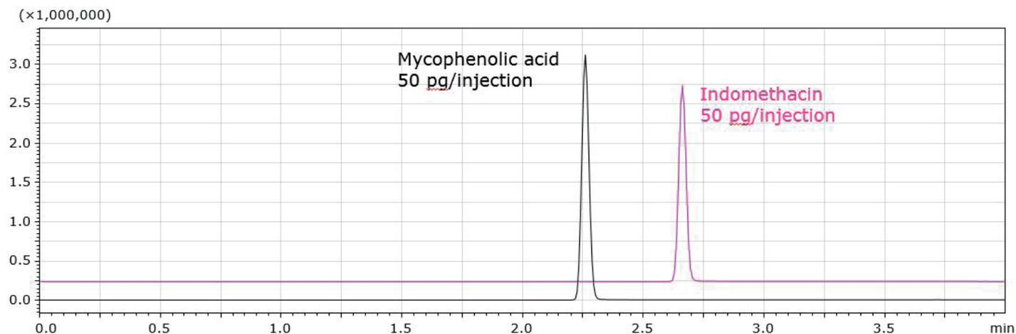
**Figure 3.** SRM chromatograms after ISOLUTE® SLE+ treatment with 5.0 µg/mL of mycophenolic acid in plasma.
