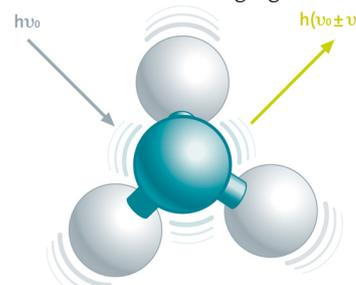
Raman effect: light interacting with chemical bonds leading to inelastic light scattering.
