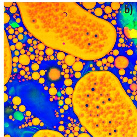
Figure 4: a) Analyzed Raman spectra of the emulsion. b) Example 2D image c) Three-dimensional confocal Raman image of the emulsion: Alkane (green), water (blue) and  $\text{CCl}_4$  + oil (yellow). Image parameters:  $200 \times 200 \times 20$  pixels,  $100 \times 100 \times 10 \mu\text{m}^3$  scan area; 0.06 s integration time per spectrum, 532 nm excitation laser.
