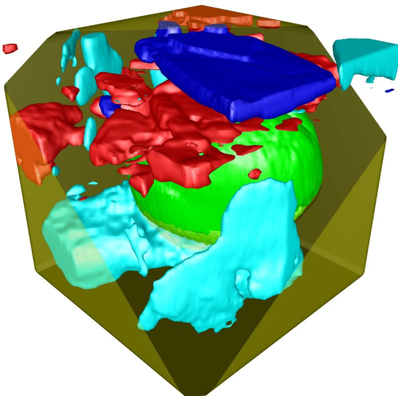
Figure 3: 3D color-coded Raman image of pollen in honey. Green: Pollen; Red, Blue, Cyan: Different crystalline phases in the honey; Yellow: Honey. Image parameters: volume size:  $50 \times 50 \times 50 \mu\text{m}^3$ ;  $150 \times 150 \times 50 = 1,125,000$  spectra; Integration time per spectrum: 2 ms.
