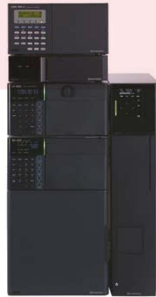
Picture 1: HIC-ESP ion chromatograph for anion detection in drinking water
