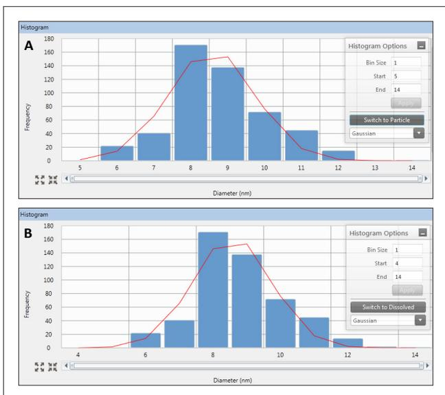
Figure 5. Size distribution histograms for NIST 8011 10 nm Au NPs using an ionic/dissolved calibration (A) and particle calibration (B).
