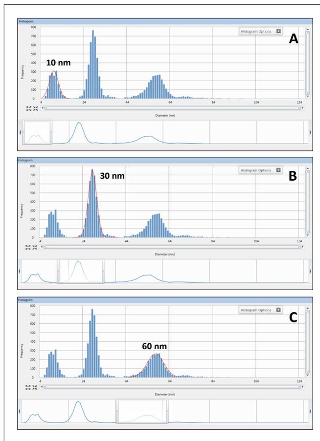
Figure 6. Size distribution histograms for a mixture of 10, 30, and 60 nm Au NPs. This average particle size determined from integrating each peak is shown on the histogram. Integration of the: 10 nm peak (A); 30 nm peak (B); 60 nm peak (C).
