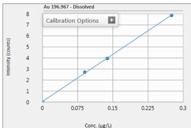
Figure 1. Dissolved calibration plot for 0.080, 0.125, and 0.275  $\mu$ g/L Au.
