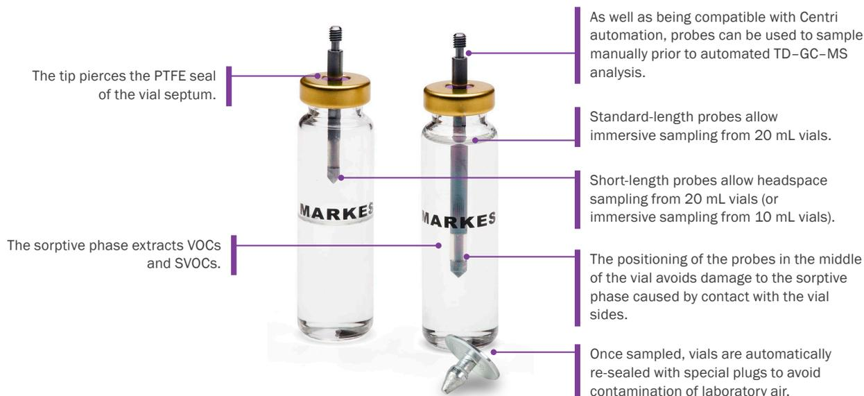
**Figure 1:** Headspace (left) and Immersive (right) sampling with HiSorb probes.
