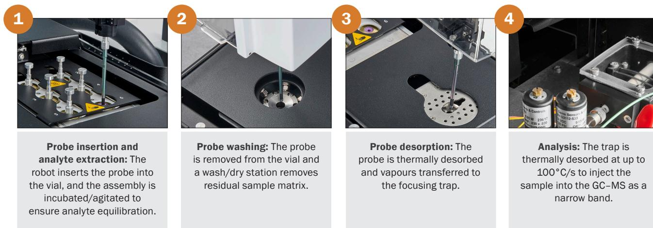
**Figure 2:** The main steps of HiSorb sampling using Centri.
