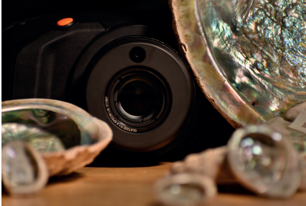
Hyperspectral camera used to record the spectrum of nacre. Courtesy of Mikhail Kats.
