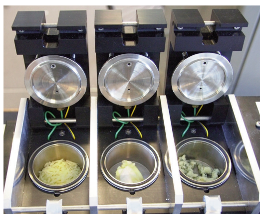
Figure 1: The Micro-Chamber/Thermal Extractor with cheese samples in place.
