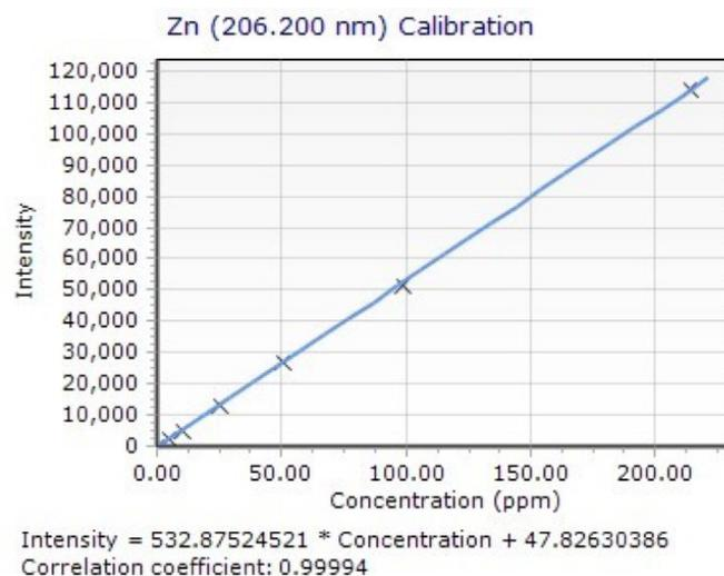
**Figure 2.** Calibration graph for Zn using the 206.200 nm emission line.
