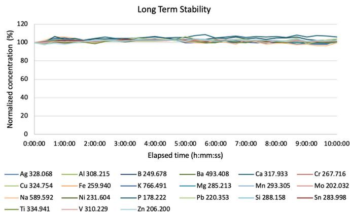
**Figure 3.** Long-term stability: recoveries of a 5 mg/kg organometallic calibration standard analyzed over the course of the 10-hour sequence.
