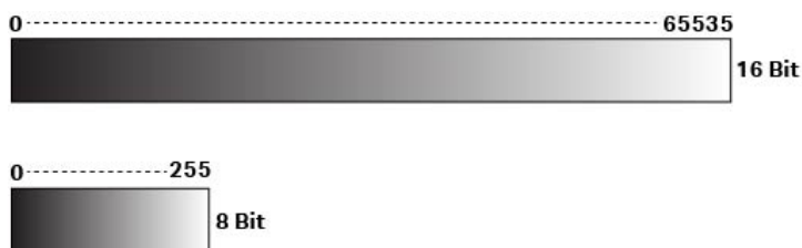
Fig 2. Grayscale .TIF files are composed of different levels of gray shades. 16-bit files have a higher number of gray scale levels than 8-bit files.
