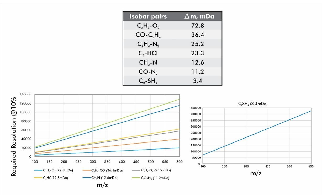
Figure 5. Required resolving power for separating various isobars.
