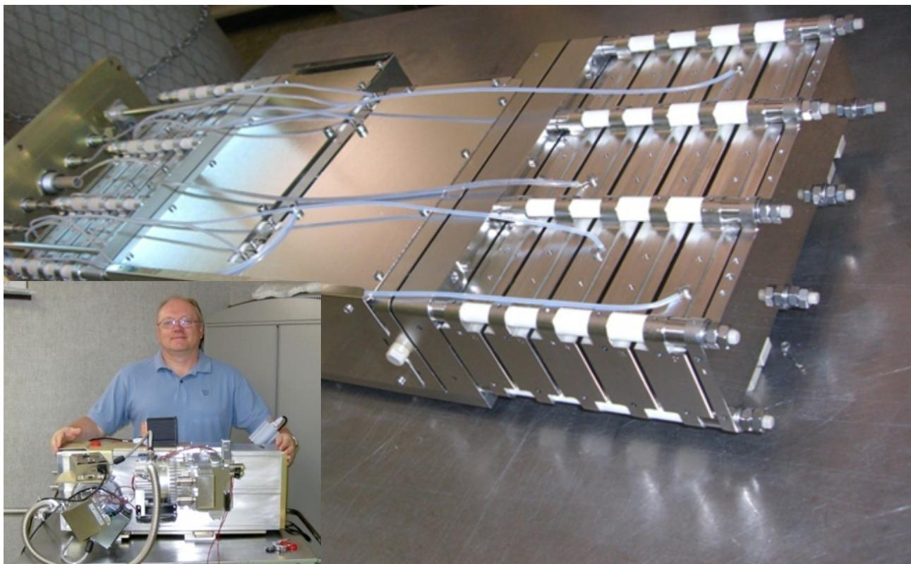
*Figure 13. An example of the FFP mass analyzer design. Inset with author for scale.*
