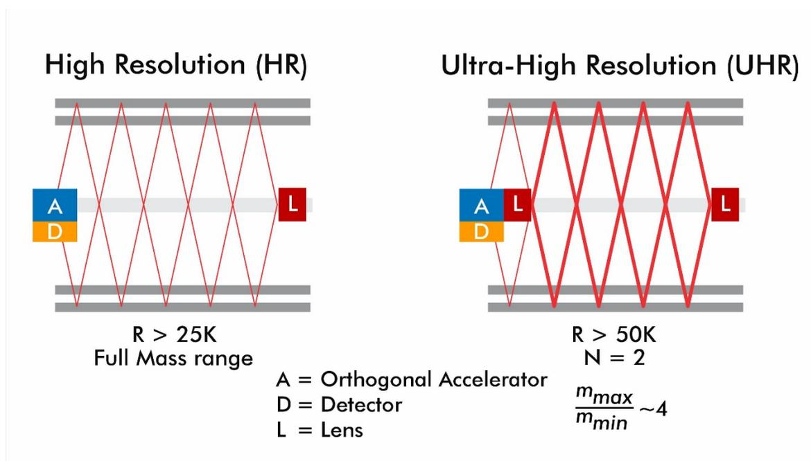
Figure 17. Modes of operation of the FFP mass analyzer: High Resolution (HR) mode (left) and Ultra-High Resolution (UHR) mode.
