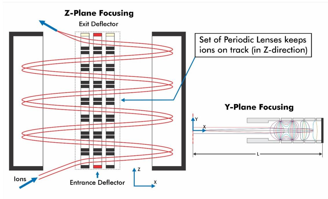
Figure 10. Design concept of the TOF mass analyzer with planar gridless electrostatic mirrors and lens array, placed between the mirrors.
