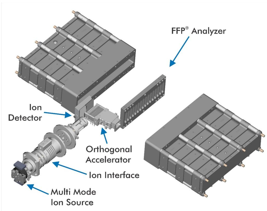
Figure 12. The ion optical CAD representation of the GC-TOFMS with FFP.
