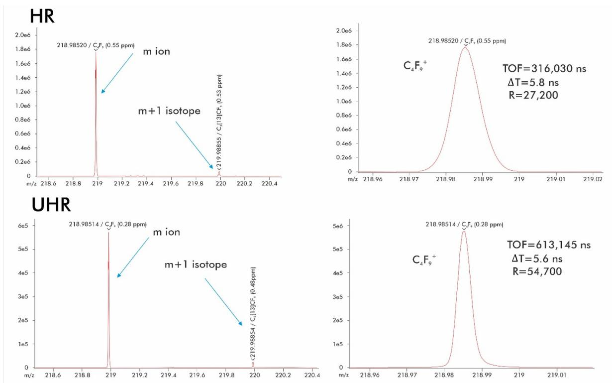
**Figure 15. Electron ionization mass spectrum of PFTBA demonstrating separation of ion fragment  $C_4F_9^+$  and its first isotope  $C_3^{13}CF_9^+$  (left) and  $C_4F_9^+$  ( $m/z=219$ ) (right) ion peak details (TOF, peak width) confirming the resolving power value above 25,000 in High Resolution (HR) mode (top) and confirming the resolving power value above 50,000 in Ultra High Resolution (UHR) mode (bottom).**
