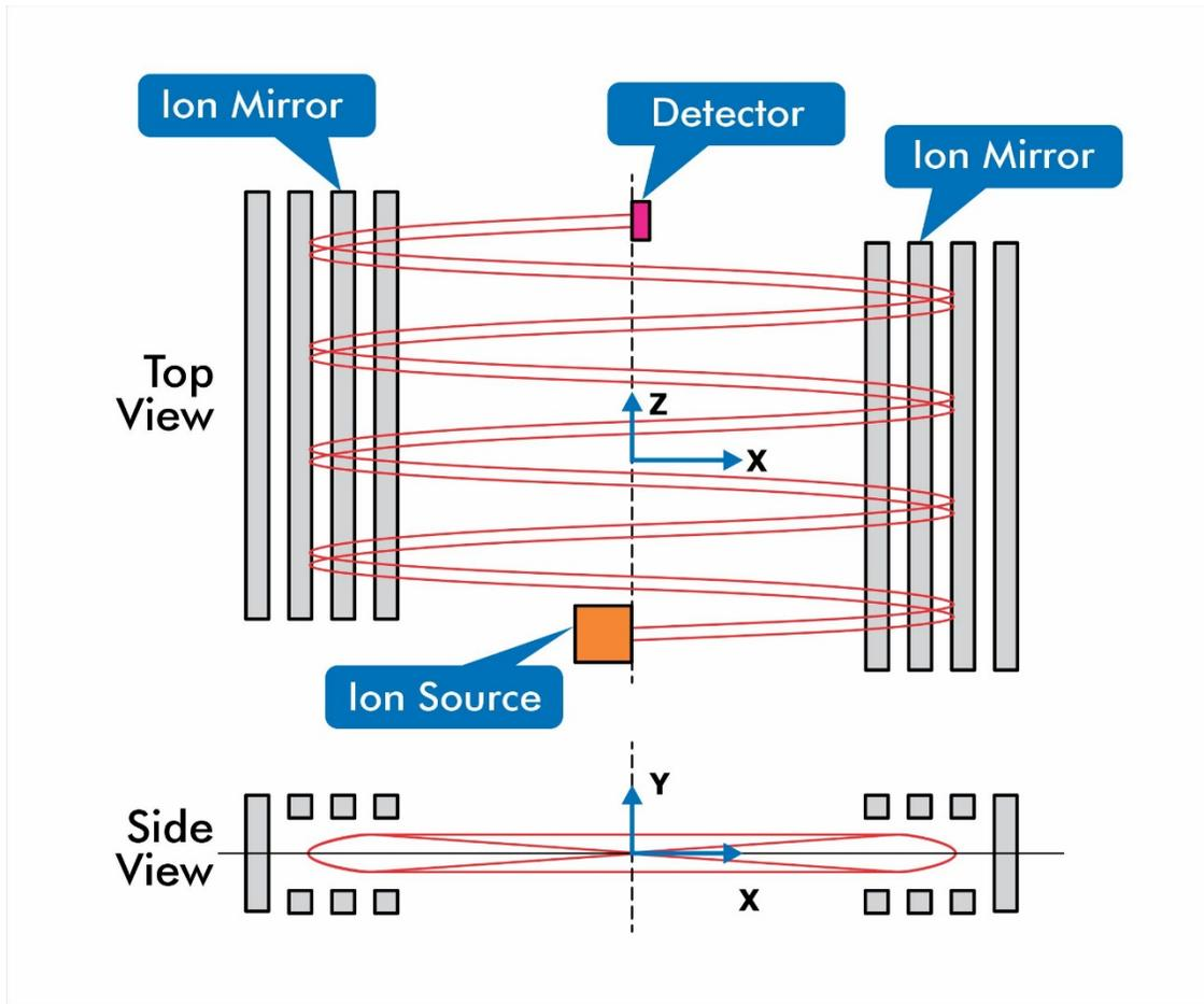
Figure 9. Design concept of the TOF mass analyzer with planar gridless electrostatic mirrors<sup>[7]</sup>.
