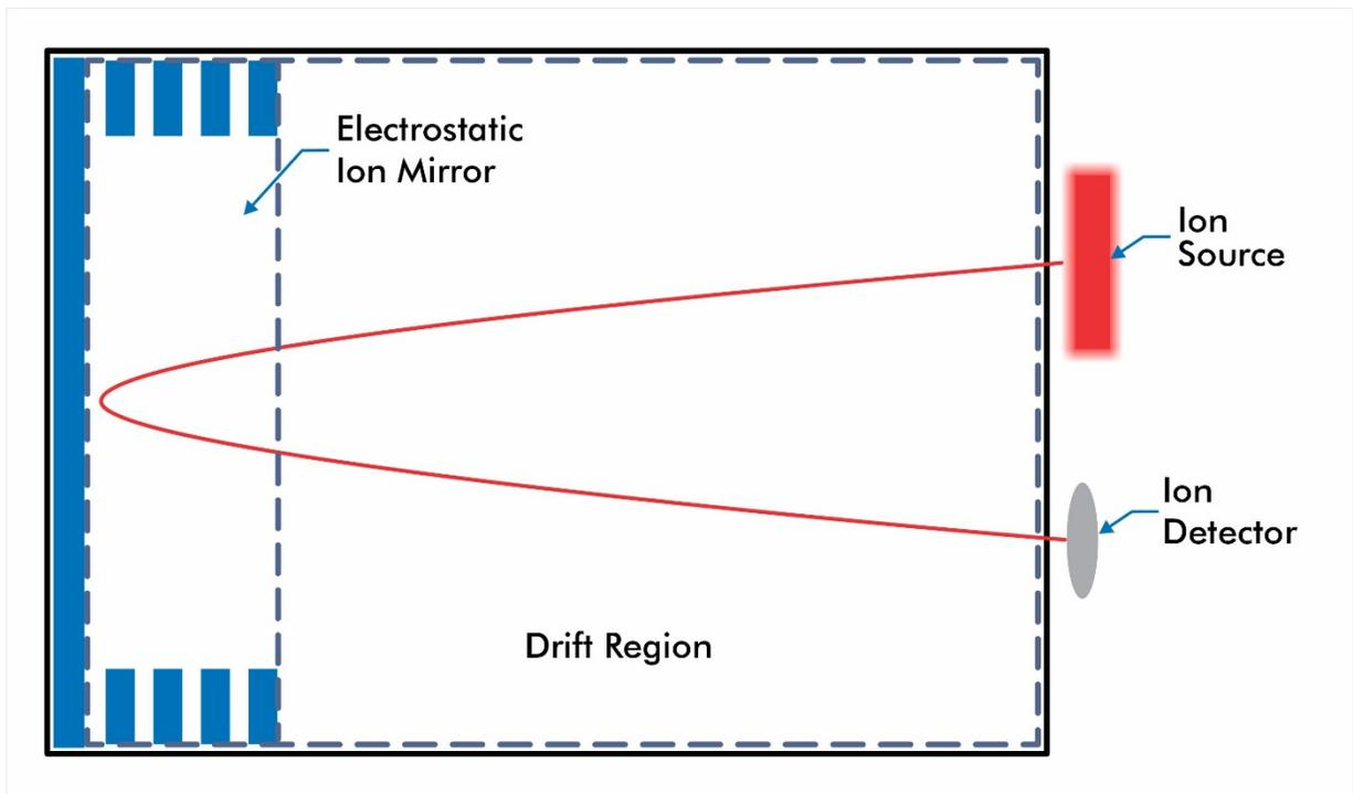
Figure 6. Reflectron mass analyzer concept.
