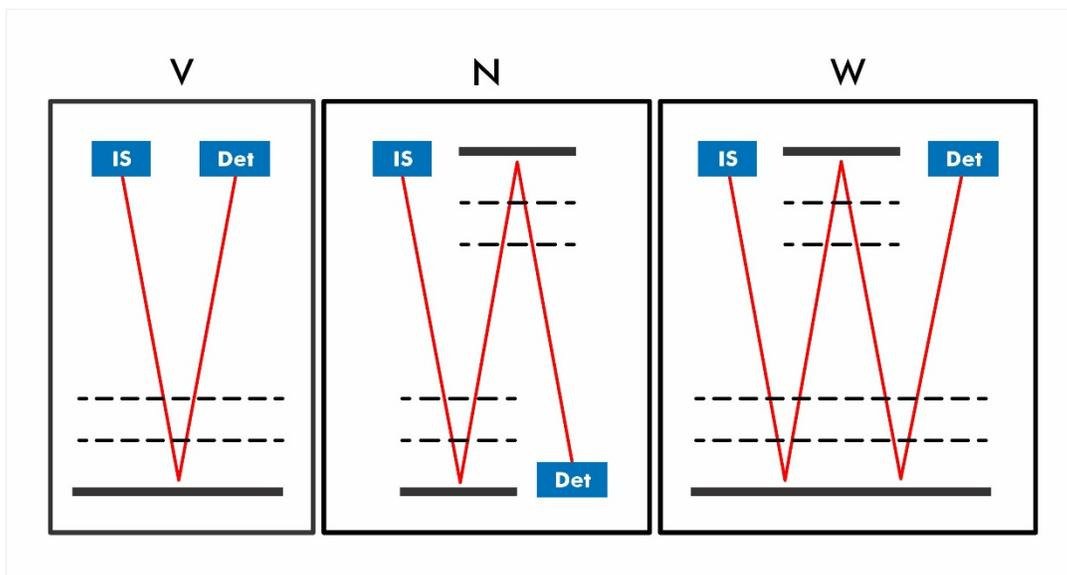
Figure 8. Reflectron analyzers configurations: V-shaped ion trajectory with a single reflection, N-shaped with two reflections, and W-shaped with three reflections. IS – Ion Source, Det – Ion Detector.
