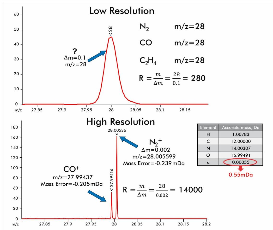
Figure 3. The effect of low vs high resolution on identification.
