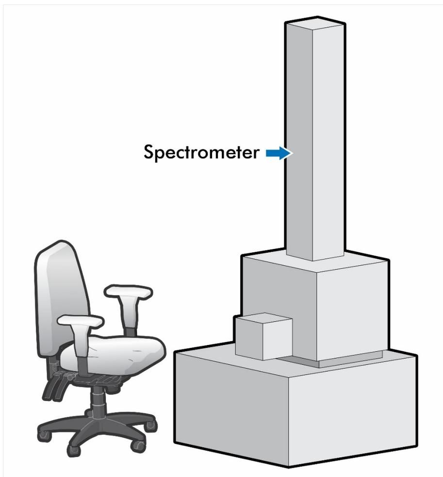
Figure 7. Increased height of the flight tube in a typical high resolution TOFMS.
