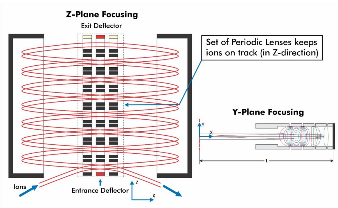
Figure 11. Folded Flight Path TOF mass analyzer concept.
