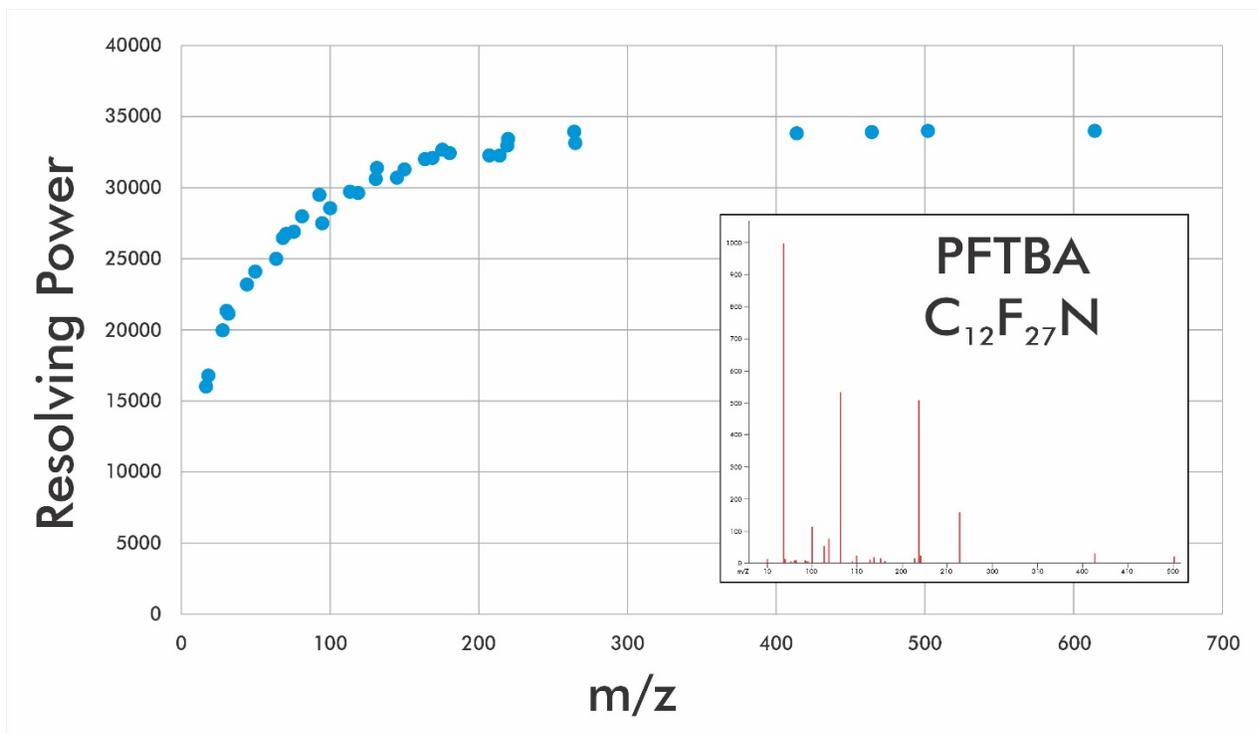
Figure 16. FFP experimental data showing resolving power vs ions' m/z obtained using GC-HRT.
