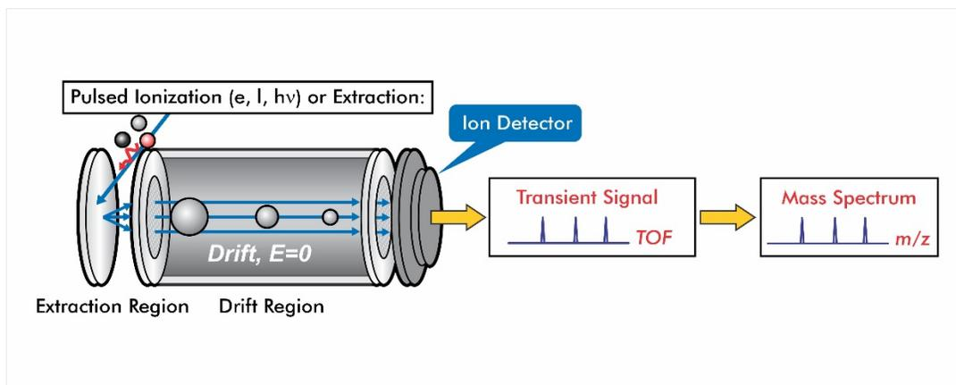
Figure 1. Time-of-flight mass spectrometer concept.
