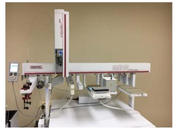
Figure 1. GERSTEL MultiPurpose Sampler (MPS robotic<sup>pro</sup>) with GERSTEL ITSP Option.
