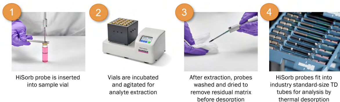
Figure 2: HiSorb sampling and analysis workflow.
