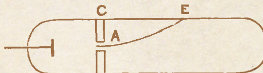
Two of Thomson's apparatus, circa 1897, to determine if cathode rays were 'negatively electrified particles'. This was a refinement of Perrin's earlier work in which he observed that negatively charged particles were influenced by the presence of a magnetic field. Ref: J. J. Thomson, "Cathode Rays", Philosophical Magazine, 44(5) 293-316 (1897).
