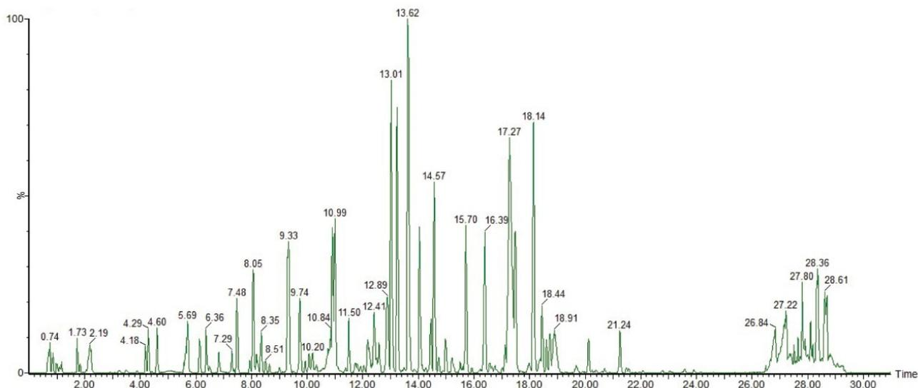
Figure 2. BPI chromatogram of tryptic digest of ENBREL (etanercept) analyzed via RPLC/HDMS<sup>E</sup> (single pass IMS).
