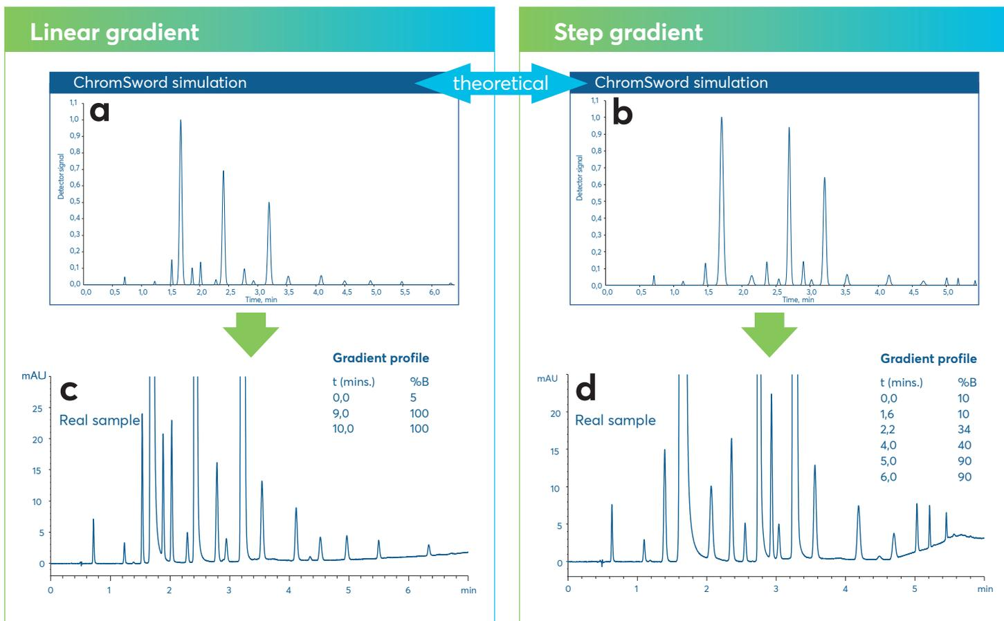
**FIGURE 3:** Simulated and experimental results from optimisation of the separation in Figure 2 by ChromSword® 2; a) predicted linear gradient separation, b) predicted step-gradient separation, c) real life chromatogram for the gradient in a and d) real life chromatogram for the step gradient in b.
