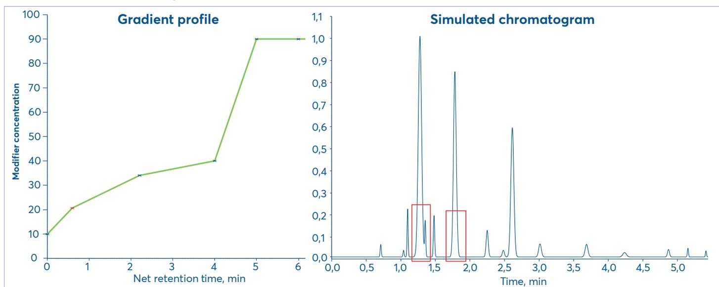
edit the gradient profile in any way desired and the corresponding chromatogram is automatically simulated (Figure 4).
