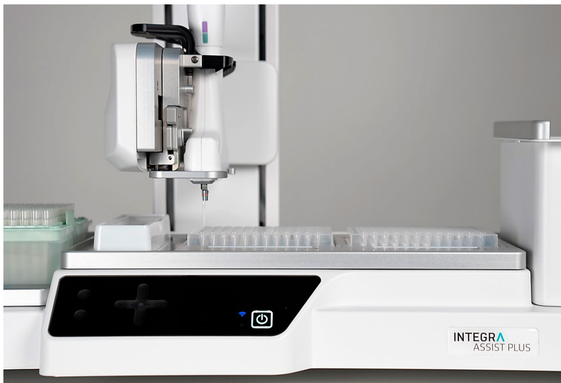
Figure 6: The D-ONE single channel pipetting module transfers the samples individually.
