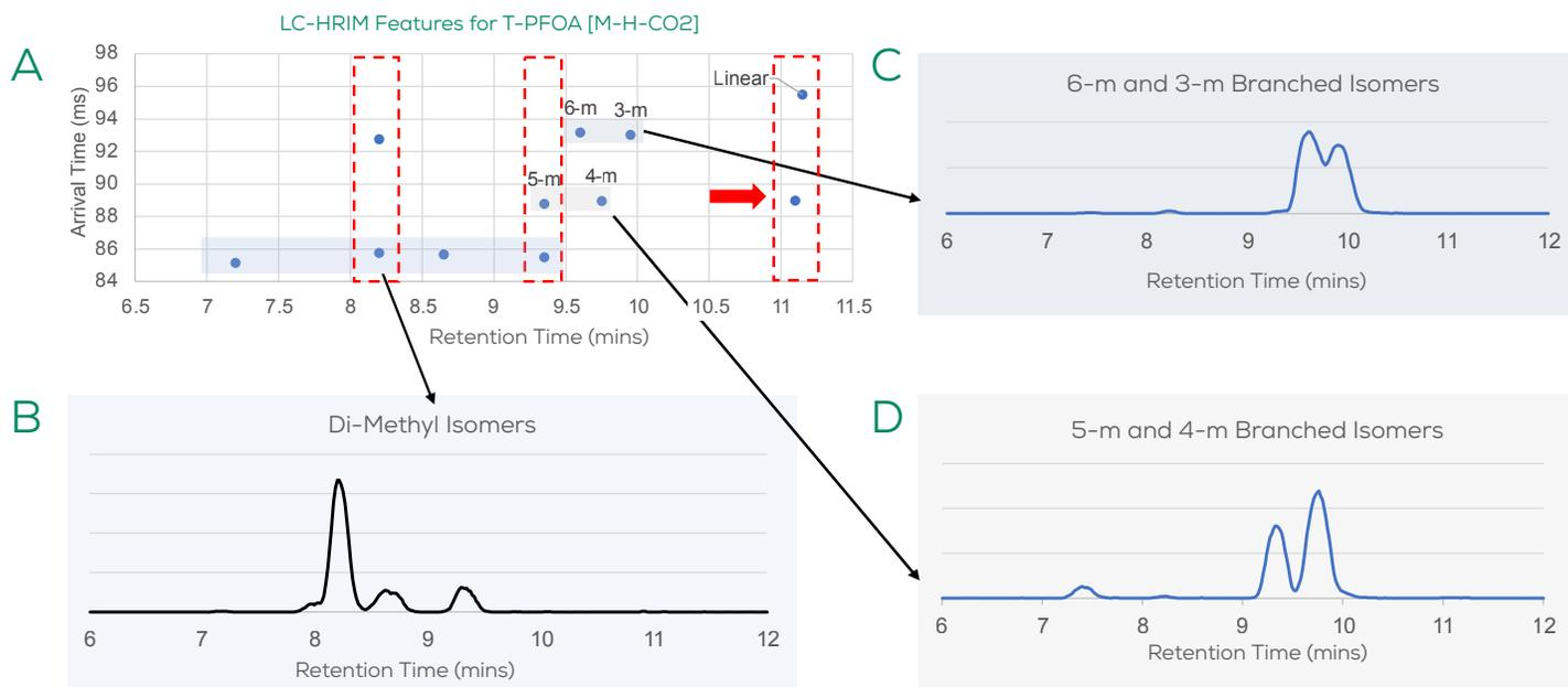
**Figure 1.** (A) Two-dimensional plot of chromatographic retention time versus the HRIM arrival time measure demonstrating complete separation of all 11 isomers in the T-PFOA standard. Red dashed boxes indicate three observed regions of the chromatogram where unresolvable compounds would reside in the absence of HRIM, with the red arrow highlighting a branched isomer in line with the linear form. (B-D) Mobility filtered extracted ion chromatograms (EICs) from the shaded regions of the 2D plot.
