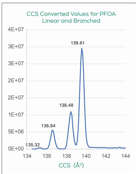
**Figure 2.** Ion mobiligram of a flow injection analysis with CCS calibration using Agilent reference mass solution.
